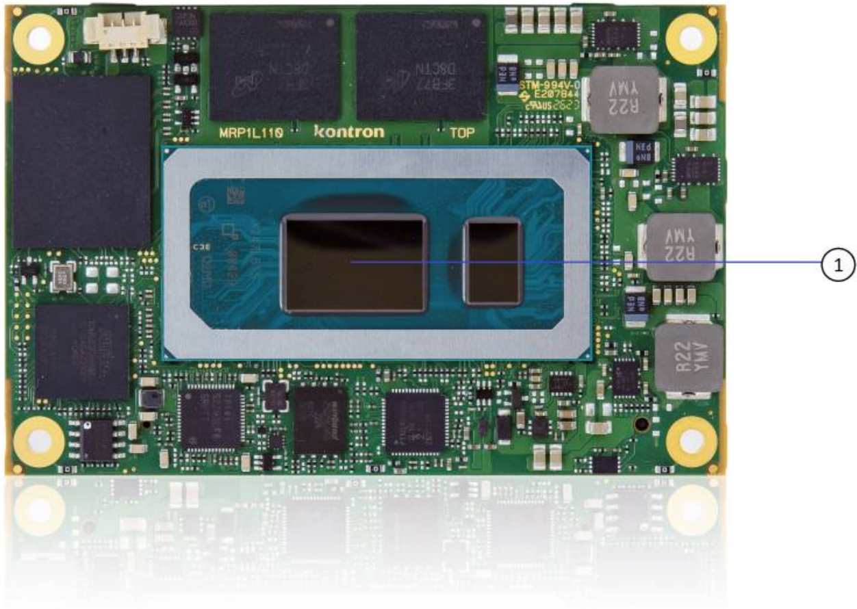
Figure 4: 1. Temperature Sensor in Processor (CPU)
