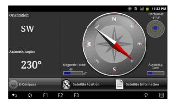
The Magnetic Field and Accuracy readings are for your reference. When the application determines that calibration is needed, it will pop up the "Calibration" graphics asking you to calibrate the compass (unless you have disabled the function). Hold the device and swing it in the way as shown on the screen. Do this several times until the popup graphics disappear.
