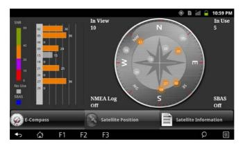
SBAS (satellite-based augmentation system) provides additional accuracy and reliability for the GPS devices. Ground stations are necessary to achieve the purpose. The SBAS feature works where such stations exist. You can enable the SBAS feature. (See "Getac Peripheral Settings" in Chapter 9.)
