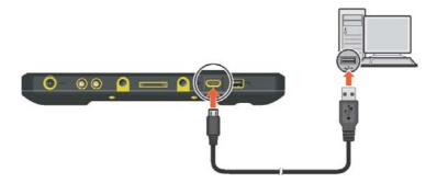
Use the USB cable (available to you as an option) to connect the device to a USB port on your computer.
