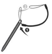
Insert the other loop end to the right-side holder on the device (as indicated by • below). Then, insert the stylus end through the loop (as indicated by • below) and pull it tight.
