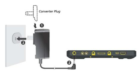
3. The charge indicator glows in amber when charging is in progress. Do not disconnect your device from AC power until the battery is fully charged, as indicated by the amber indicator turning into green. This will take a couple of hours.
