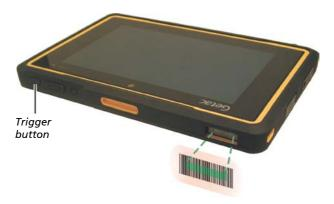
**NOTE:** If the code being scanned is highly reflective (e.g., laminated), it may be necessary to tilt the code +5° to prevent unwanted reflection.
